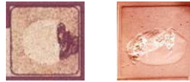
Fig 2. Photos of bond pads w/ contamination that prevented good intermetallics and led to ball lifting
