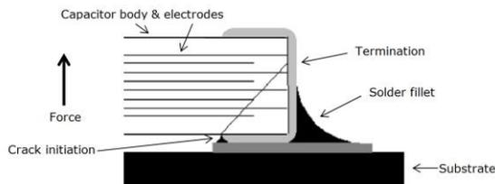
Example of capacitor issued by customers to Knowles Precision Devices for failure investigation:
