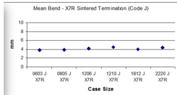
It can be seen that mean bend distance achieved by Class I COG/NP0 (1B/CG) is typically 7mm while Class II dielectrics have a mean value of typically 4mm.
