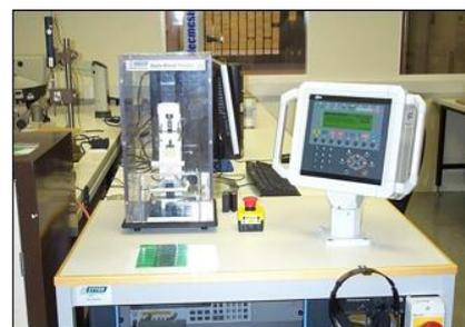
Figure 9 shows the bend test fixture, the hardened steel press head is programmed to follow a deflection profile, with a ramp rate of 1mm/s and dwells in accordance with AEC-Q200-005
