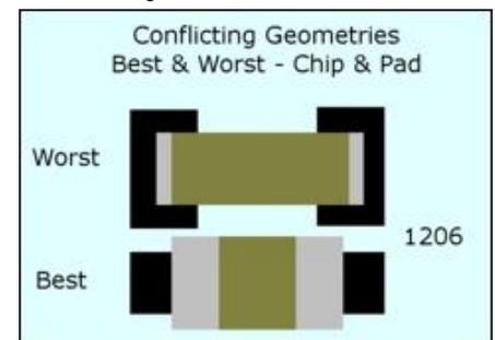
Figure 5 gives guidance on the pad/ land size to capacitor component to reduce the likelihood of mechanical damage.
