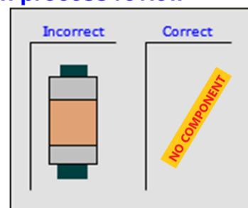
flexing of the PCB creates mechanical stress within the capacitor that if sufficient can result in the capacitor being mechanically cracked.
