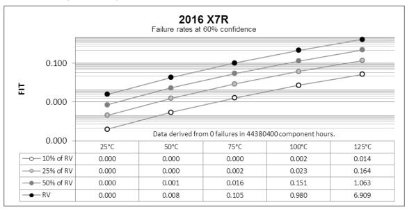
The FIT (Failure In Time) rate graph provides an indication of component reliability in relation to a customer's application with respect to temperature and voltage being applied. For example, at 25°C and 50%RV (Rated Voltage), the FIT rate graph indicates 0.000 FITs. As a comparison, an automotive customer specifies maximum of 0.1 FITs at 25°C and 50%RV (Rated Voltage).
