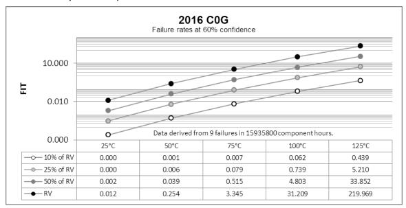
The FIT (Failure In Time) rate graph provides an indication of component reliability in relation to a customer's application with respect to temperature and voltage being applied. For example, at 25°C and 50%RV (Rated Voltage), the FIT rate graph indicates 0.002 FITs.
