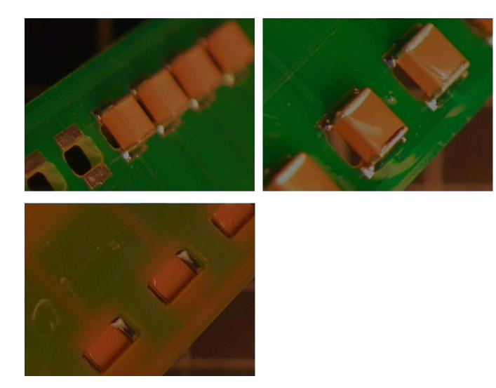
The boards should be routed out completely between the opposing pads and extending either side of the MLCC, so no part of the MLCC beyond the soldered areas is in contact with the board surface.
