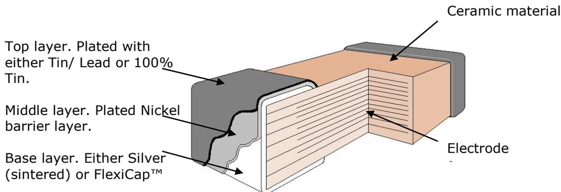
Figure 1 - Capacitor construction diagram
