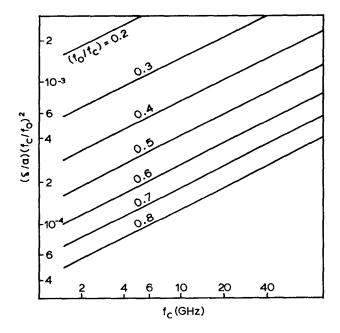
Fig. 3. Plot of  $(\delta/a)(f_c/f_o)^2$  vs.  $f_c$  for brass waveguide.
