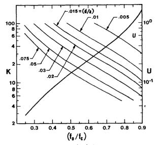
Fig. 2. Curves of K vs.  $(f_o/f_c)$  of the TE<sub>01</sub> mode.
