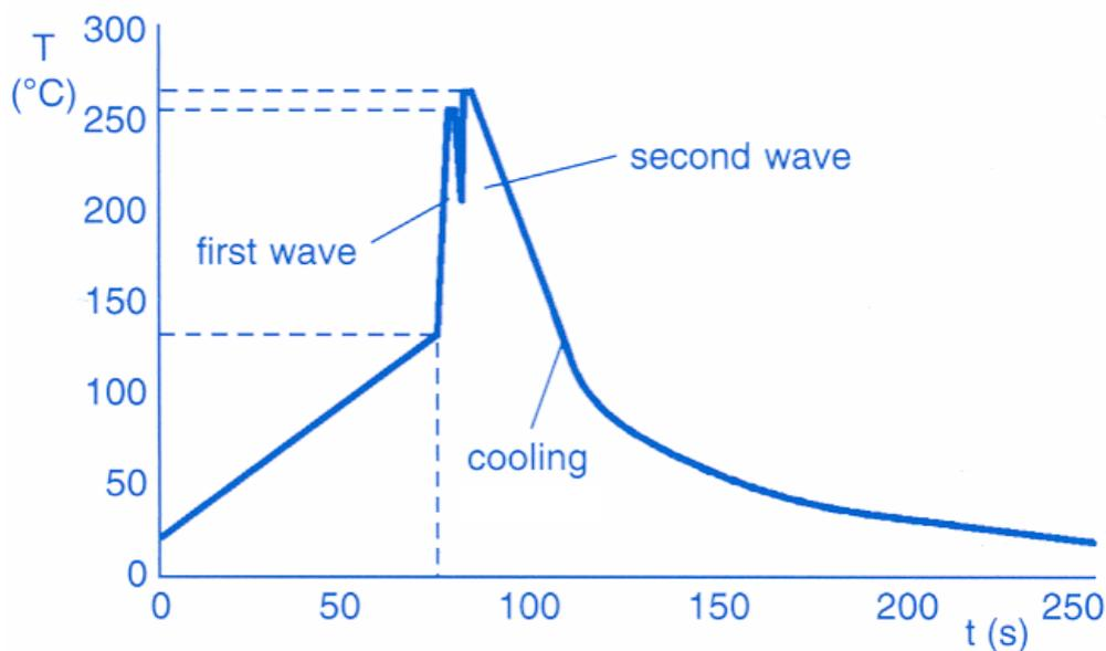
Maximum permissible wave temperature is 270°C for SM chips and 260°C for Radial Leaded capacitors – see also note above regarding radial leaded capacitors.
