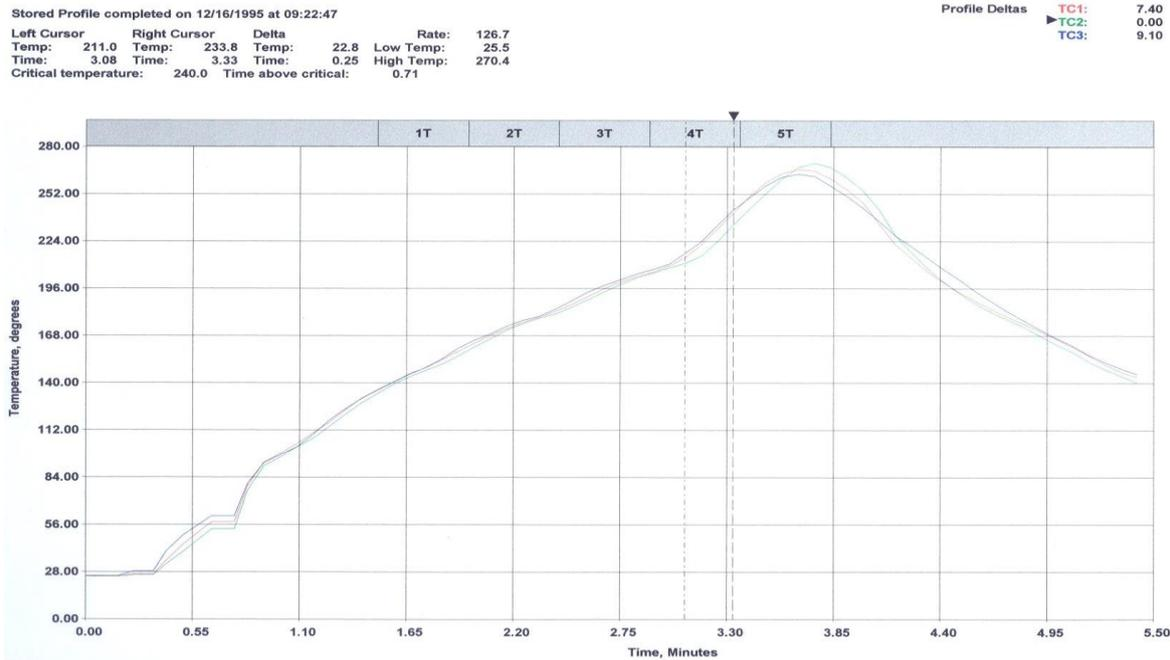
When discussing a reflow profile, we can only give a general recommendation as to the shape of the profile. We cannot give a definitive profile of the actual peak temperatures, as this is dependant on a number of factors which can only be decided by the assembler – the type of solder used, the size, specification and arrangement of other components on the board and the overall thermal mass of the board.
