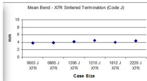
It can be seen that mean bend distance achieved by Class I C0G/NP0 (1B/CG) is typically 7mm while Class II dielectrics have a mean value of typically 4mm.
