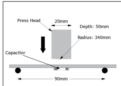
Devices Test PCBs are mounted with one capacitor and deflected automatically until the capacitor breaks. The software analyses the change in capacitance measured by the Agilent 4288A capacitance meter. As soon as the capacitance change is greater than 10% the bend deflection distance is recorded in millimetres. The maximum deflection of the machine is 10mm.
