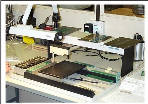
The PCB are then subjected to bend testing in accordance AEC-Q200-005 using Knowles Precision Devices purpose build bend test facility, Figure 8.
