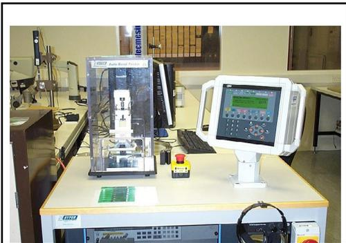
Figure 9 shows the bend test fixture, the hardened steel press head is programmed to follow a deflection profile, with a ramp rate of 1mm/s and dwells in accordance with AEQ-Q200-005
