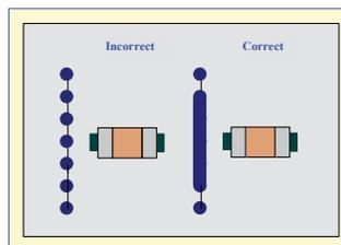
Figure 5 gives guidance on the pad/ land size to capacitor component to reduce the likelihood of mechanical damage.
