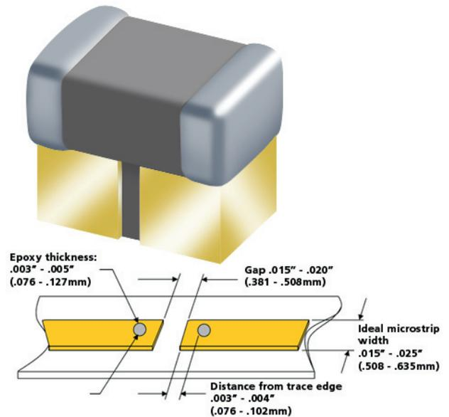
4. After the reflow step is completed, inspect joint for voids or excess flux and non-reflowed solder balls that can degrade performance or cause shorts across the gaps. Proper cleaning after the reflow process is crucial to avoiding performance degradation and discovering poor solder joints.
