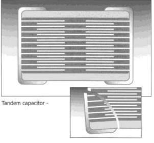
Qualification of both Open Mode and Tandem included cracking the components by severe bend tests. Following the bend tests cracked components were subjected to endurance/ humidity tests, with no failures evident due to short circuits. Note: Depending on the severity of the crack, capacitance loss was between 0% and 50%.
