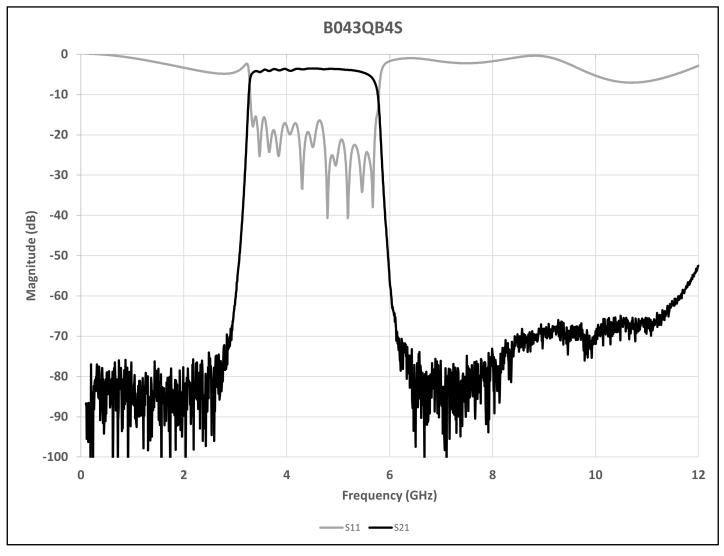
\*Typical de-embedded measured performance mounted on a connectorized test fixture. DEB is 0.010in RO4350B with 50.00hm CPW ground traces going into the ports at room temperature.
