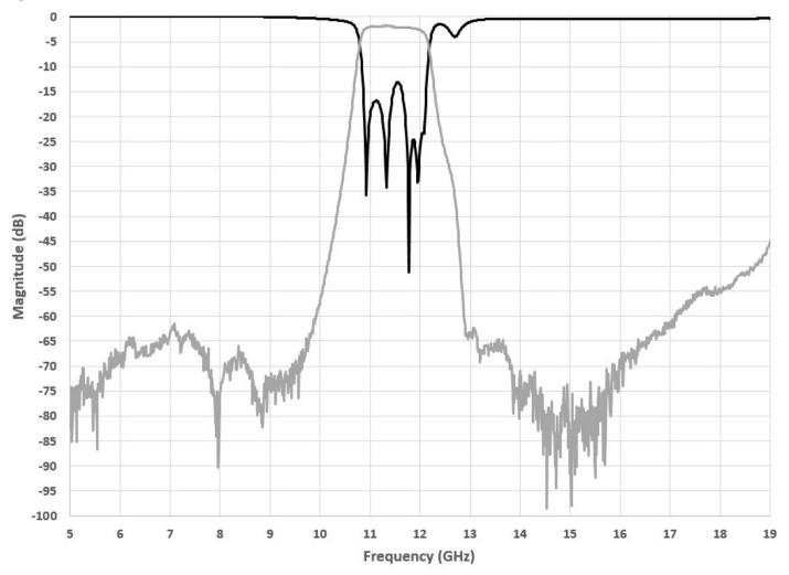
\*Typical de-embedded measured performance mounted on a connectorized test DEB (0.010in RO4350B with 50 $\Omega$  CPW ground traces), tested at room temperature
