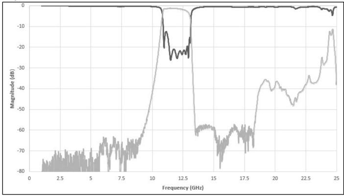
\*Typical de-embedded measured performance mounted on a connectorized test fixture. DEB is 0.010in RO4350B with 50.00hm CPW ground traces going into the ports at room temperature.
