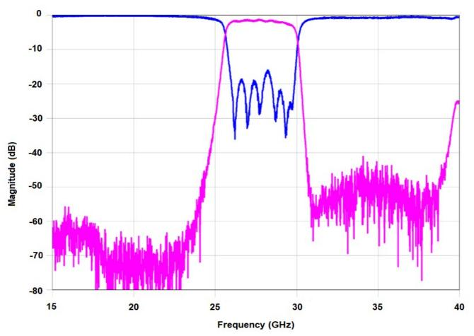
\*Typical de-embedded measured performance mounted on a connectorized test fixture. DEB is 0.010in RO4350B with 50.00hm CPW ground traces going into the ports at room temperature.
