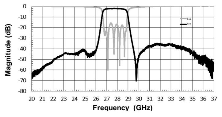
\*Typical de-embedded measured performance mounted on a connectorized test fixture. DEB is 0.010in RO4350B with 50.00hm CPW ground traces going into the ports at room temperature.
