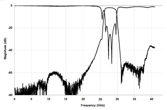
\*Typical de-embedded measured performance mounted on a connectorized test fixture. DEB is 0.010in RO4350B with 50.00hm CPW ground traces going into the ports at room temperature.
