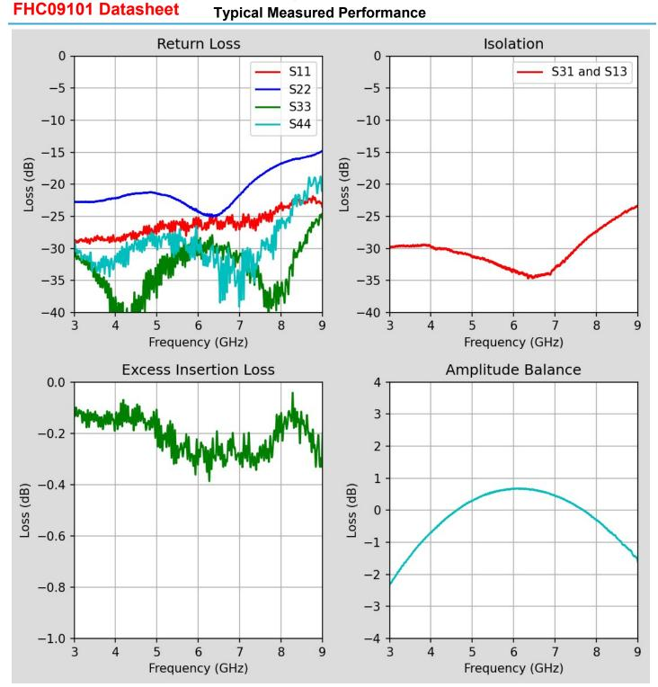
\*Typical de-embedded measured performance mounted on a connectorized test fixture. Evaluation Board is 0.010in RO4350B with 50.0 Ohm CPW ground traces going into the ports at room temperature.
