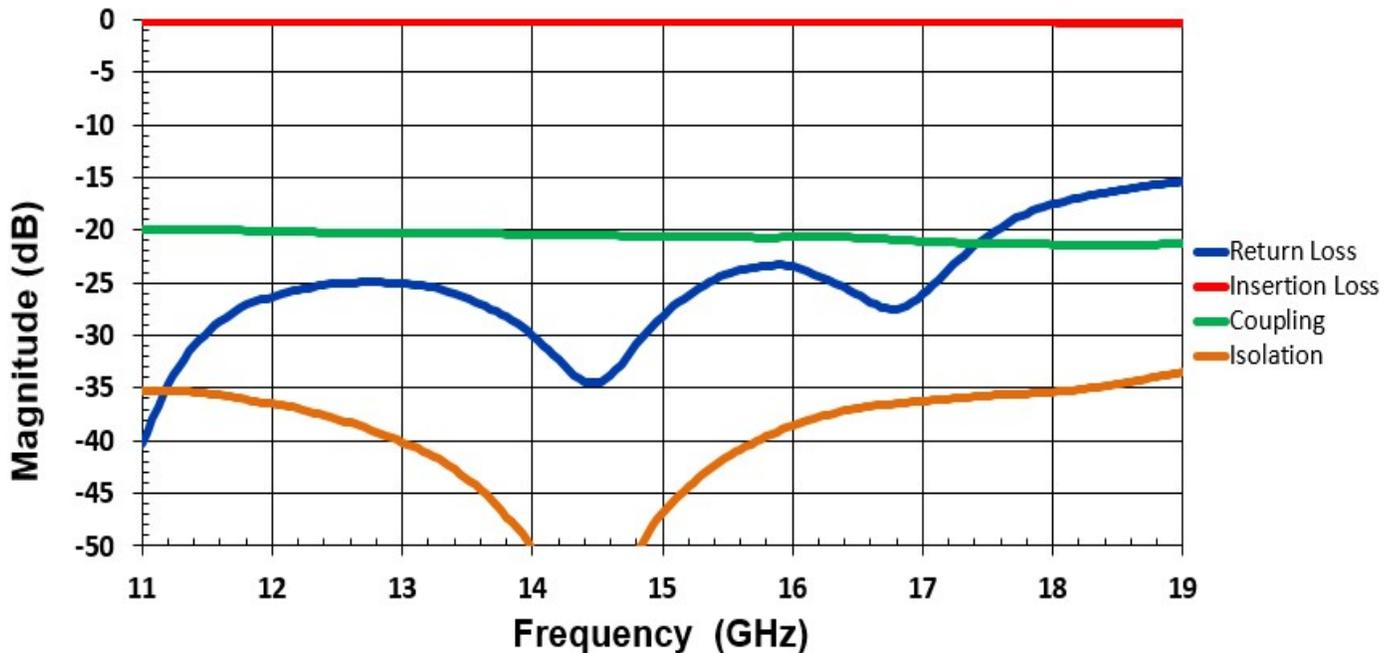
\*Typical de-embedded measured performance mounted on a connectorized test fixture. DEB is 0.010in RO4350B with 50.00ohm CPW ground traces going into the ports at room temperature.
