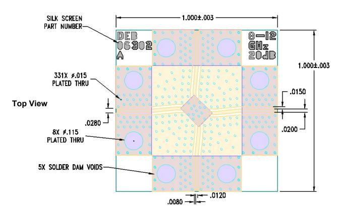
The CPWG traces going into the ports have been tapered at the board edge to accommodate capacitive loading of the Southwest connector's center pin
