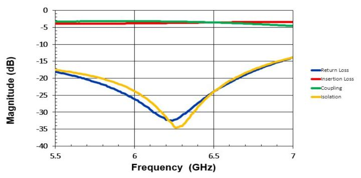
\*Typical de-embedded measured performance mounted on a connectorized test fixture. DEB is 0.010in RO4350B with 50.00hm CPW ground traces going into the ports at room temperature.
