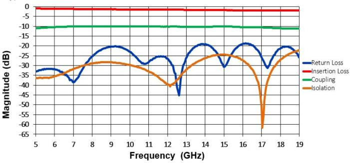
\*Typical de-embedded measured performance mounted on a connectorized test fixture. DEB is 0.010in RO4350B with 50.00hm CPW ground traces going into the ports at room temperature.
