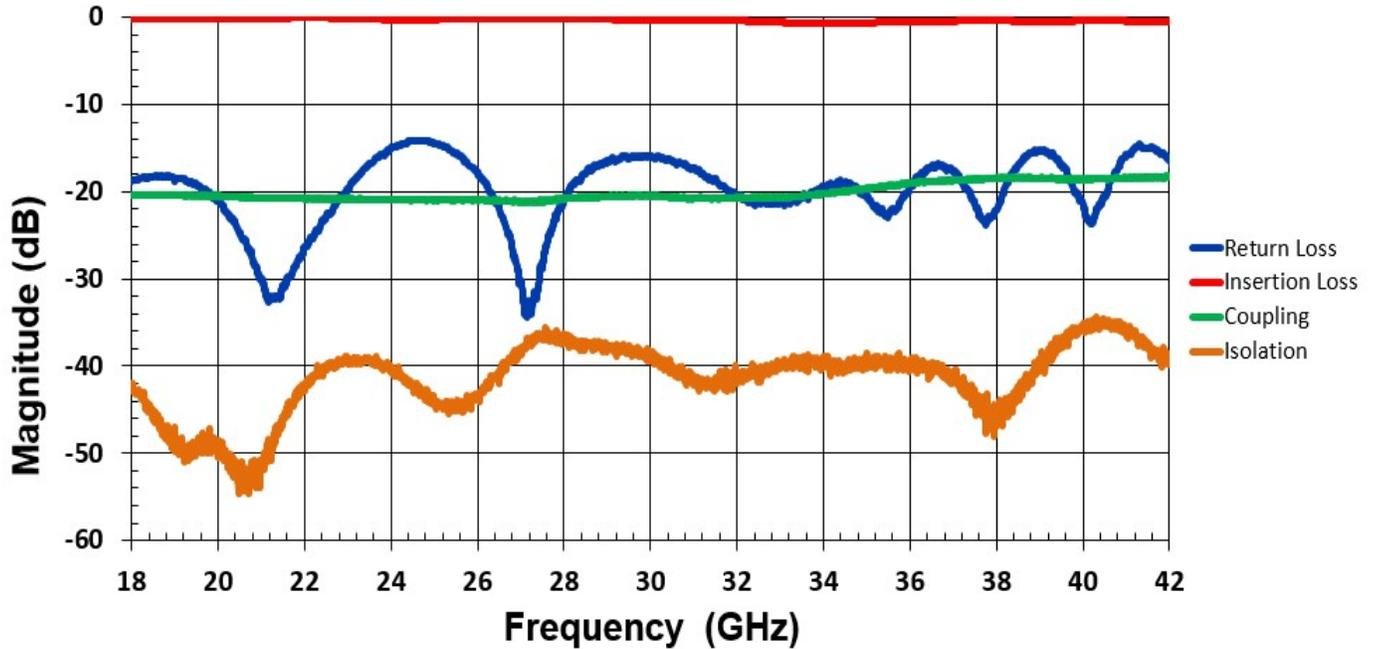
\*Typical de-embedded measured performance mounted on a connectorized test fixture. DEB is 0.010in RO4350B with 50.0Ohm CPW ground traces going into the ports at room temperature.
