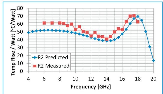
Figure 7: R2 Temperature Rise per Watt
