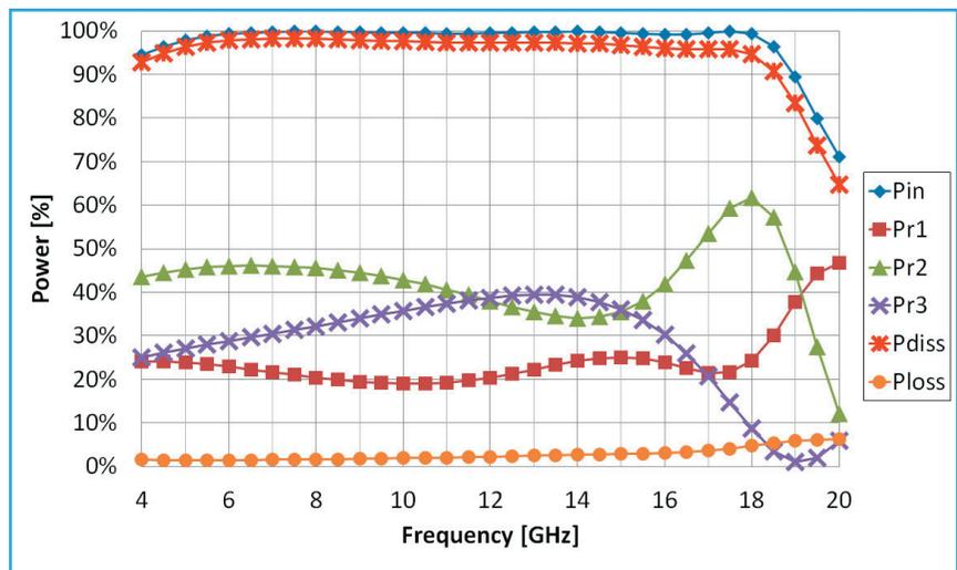
Figure 4: Power Budget for Odd Mode Excitation
