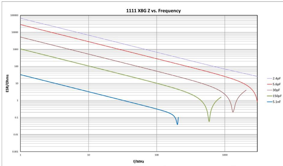
Note curves are typical, based on data measured using a Boonton 34A resonant tube and Keysight E4991 impedance analyser with Keysight 16196B/16197A test fixture.
