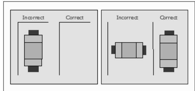
Capacitor placement not recommended in the corner of the PCB.
