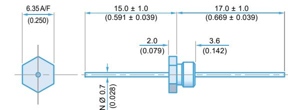
**Low Profile****M5 x 0.8 - 6g Thread****6.35mm Hexagonal Head****Electrical Details**
