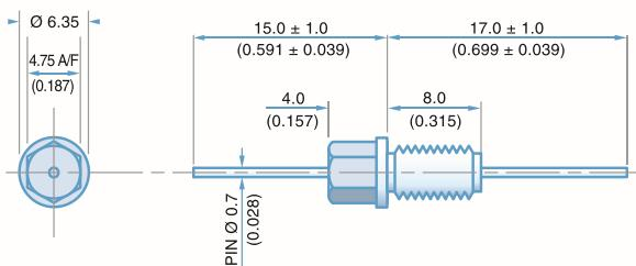
**M5 x 0.8 - 6g Thread****4.75mm Hexagonal Head/6.35mm flange****Electrical Details**
