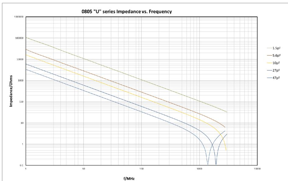
Note curves are typical, based on data measured using a Boonton 34A resonant tube and Keysight E4991 impedance analyser with Keysight 16197A test fixture
