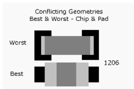
Reducing the pad/ land size can reduce the level of stress exerted onto the capacitor by approximately 50%.
