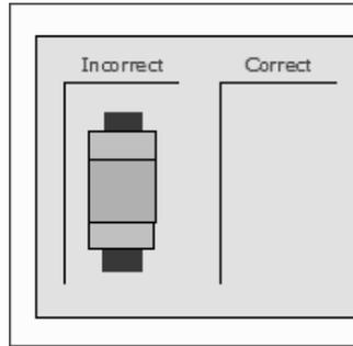
Capacitor placement not recommended in the corner of the PCB.
