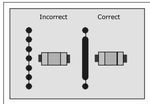
Using a slot along the depanelisation edge reduces the level of stress exerted onto the capacitor by approximately 50%.
