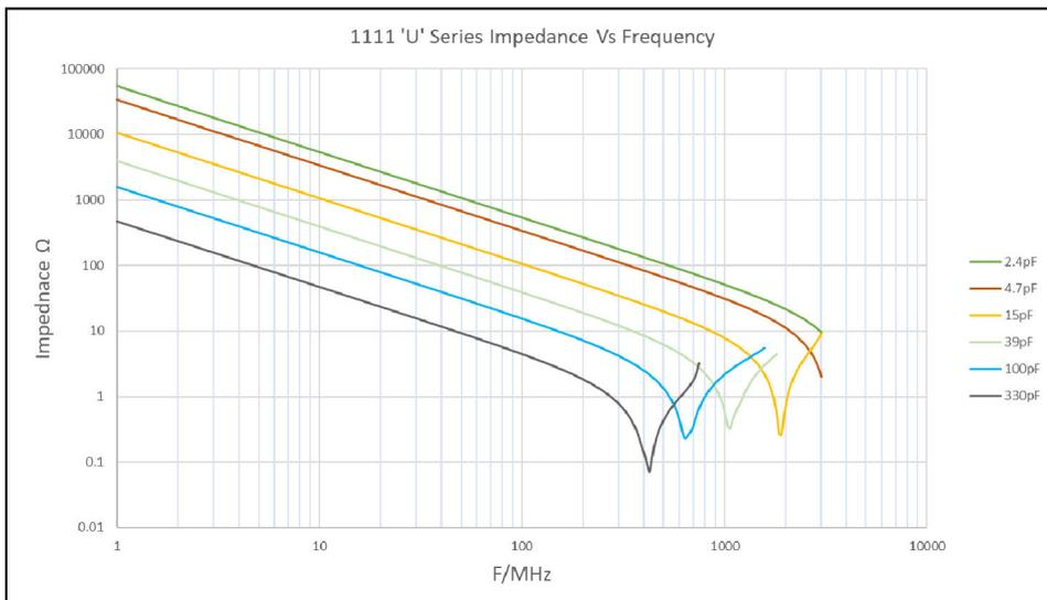
Note curves are typical, based on data measured using a Boonton 34A resonant tube and Keysight E4991 impedance analyser with Keysight 16197A test fixture
