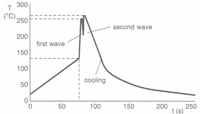
Total immersion exposure time for Sn/Ni terminations is 30s at a wave temperature of 260°C. Note that for multiple soldering operations, including the rework, the soldering time is cumulative.
