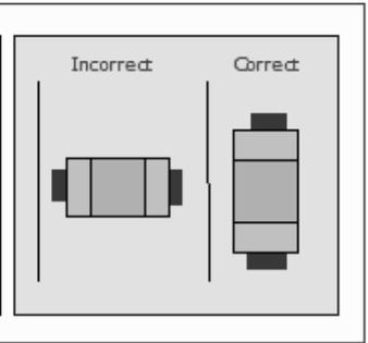
Recommended capacitor orientation with respect to PCB edge (denoted by black lines).
