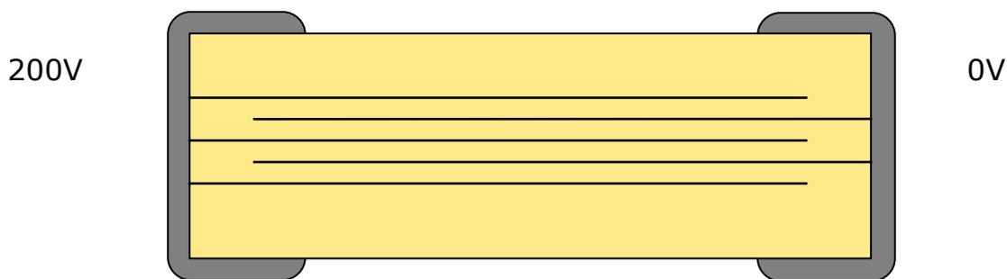
In the case of short circuit failure of this type of component, the capacitor would no longer function, and the circuit would be at risk.
