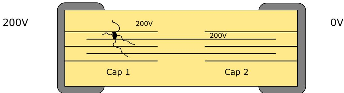
The left hand capacitor failed due to short circuit, but the right hand capacitor would continue to function as a normal capacitor, although the component capacitance would change depending on failure mechanism.
