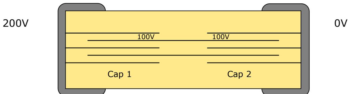
**NB** - Each section of the tandem capacitor has only 50% of the rated voltage (DWV) applied during normal use, so the component is under a low stress condition.
