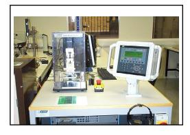
Figure 9 shows the bend test fixture, the hardened steel press head is programed to follow a deflection profile, with a ramp rate of 1mm/s and dwells in accordance with AEQ-Q200-005
