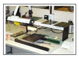
The PCB are then subjected to bend testing in accordance AEC–Q200-005 using Knowles Precision Devices purpose build bend test facility, Figure 8.
