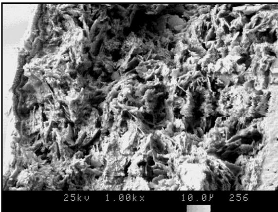
Picture taken at 1000x magnification using a SEM showing a fracture section through a capacitor termination.
