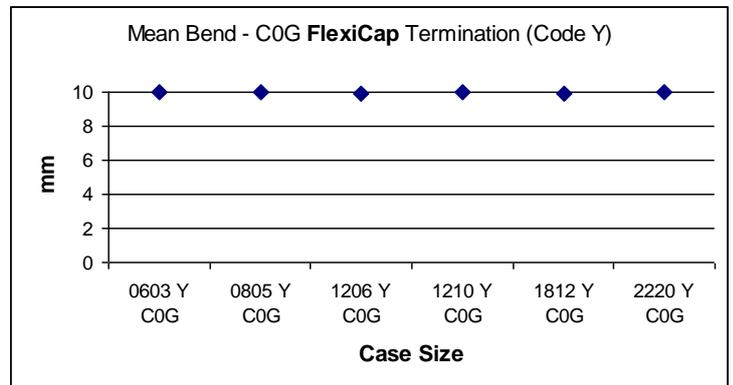
(10mm maximum bend test equipment capability)
