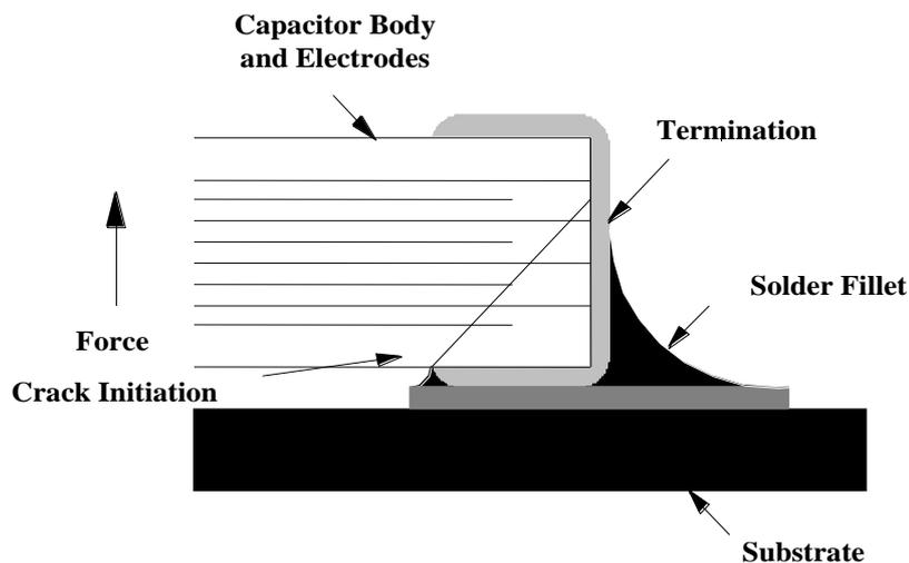
Fig 1. Mechanical Crack
