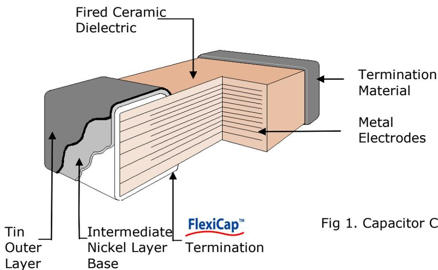
Fig 1. Capacitor Construction
