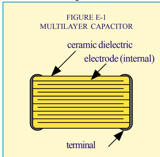
In this “multilayer” configuration, the area A is increased by virtue of many electrodes in parallel arrangement, in a construction permitting very thin dielectric thickness between opposing electrodes, such that the capacitance C is enlarged by the factor N (number of dielectric layers) and reduced dielectric thickness  $t'$ , where A' is now the area of overlap of opposing electrodes:
