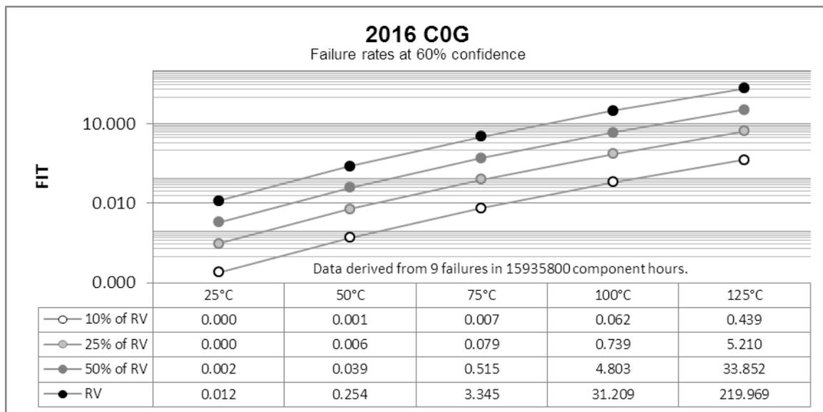
The FIT (Failure In Time) rate graph provides an indication of component reliability in relation to a customer's application with respect to temperature and voltage being applied. For example, at 25°C and 50%RV (Rated Voltage), the FIT rate graph indicates 0.002 FITs.
