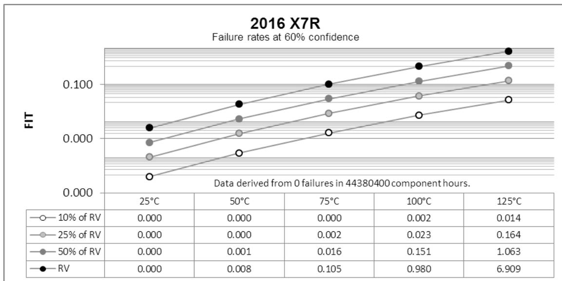
The FIT (Failure In Time) rate graph provides an indication of component reliability in relation to a customer's application with respect to temperature and voltage being applied. For example, at 25°C and 50%RV (Rated Voltage), the FIT rate graph indicates 0.000 FITs. As a comparison, an automotive customer specifies maximum of 0.1 FITs at 25°C and 50%RV (Rated Voltage).
