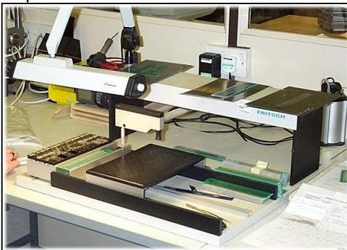
Hand pick and place used to mount capacitors for bend tests
