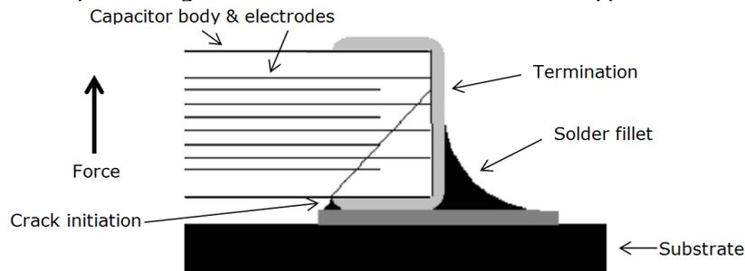
During Syfer's initial investigation into mechanical cracking over 15000 capacitors were subjected to bend testing.
