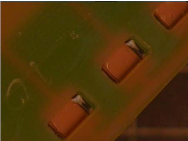
The boards should be routed out completely between the opposing pads and extending either side of the MLCC, so no part of the MLCC beyond the soldered areas is in contact with the board surface.
