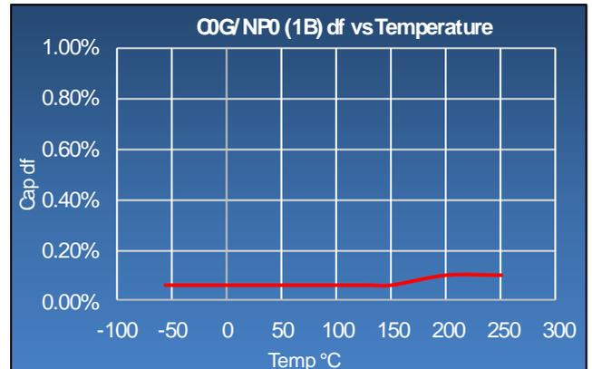
Note: 200°C COG/NPO (1B) parts life tested at maximum rated voltage and temperature for 4000Hr duration.
