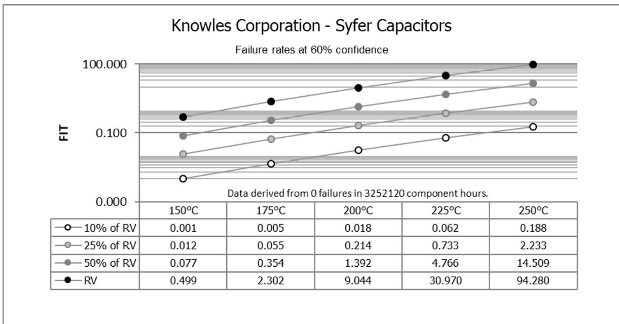
The FIT (**F**ailure **I**n **T**ime) rate graph provides an indication of component reliability in relation to a customer's application with respect to temperature and voltage being applied. For example, at 160°C and 50%RV (200°C Rated Voltage range), the FIT rate graph indicates 0.077 FITs.
