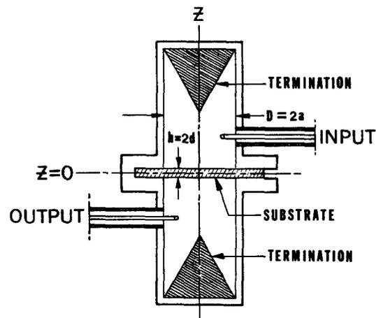
Fig. 1. Schematic cross section of substrate tester.
