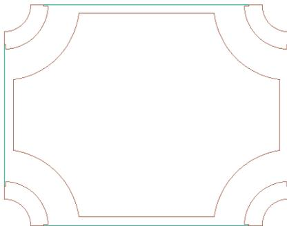
2. Window pane the ground plane targeting 70-80% area coverage with deposits of a similar size. Maintain at least 10 mils distance between the IO deposit and all ground plane deposits
