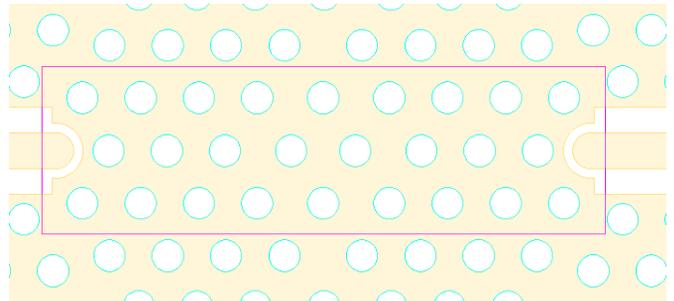
1. Make a circular deposit at each IO with a diameter matching the annular ring diameter on the bottom of the part (Figure 1)
