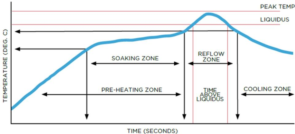
The diagram above identifies the critical parts of a reflow profile to consider for best assembly outcomes
