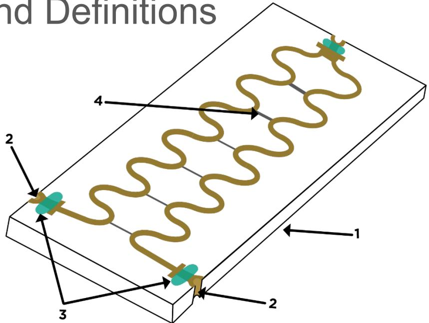
DLI brand Power Dividers can be used to divide or combine a signal. Critical areas are as follows
