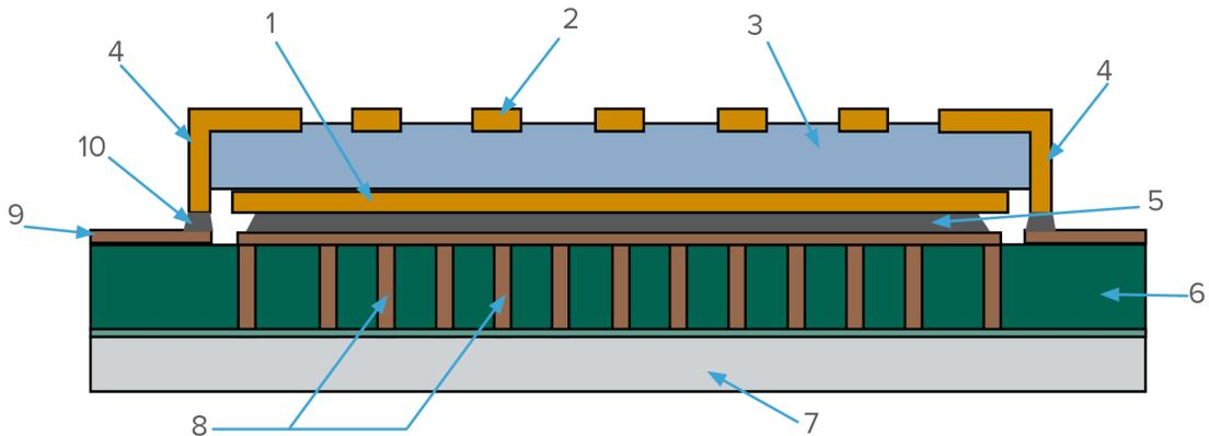
This diagram is a cross section through a surface mounted device to illustrate the necessary connections and configuration.
