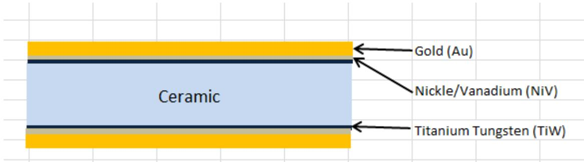
The sputtering process is much more consistent in terms of the metal layer thickness when measured across the plate. Wet Plating will typically show peaks and valleys across the plate.
