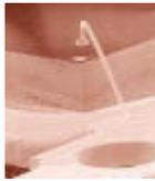
Fig 1. Photo of a lifted ball bond
